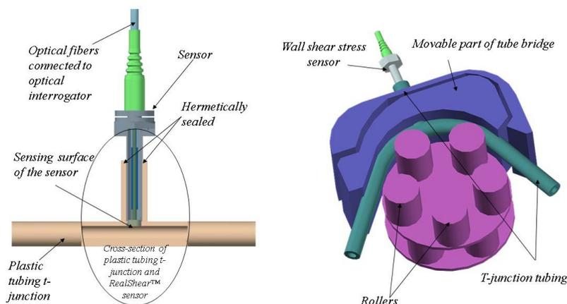
Figure 1. WSS port installed with PF6
